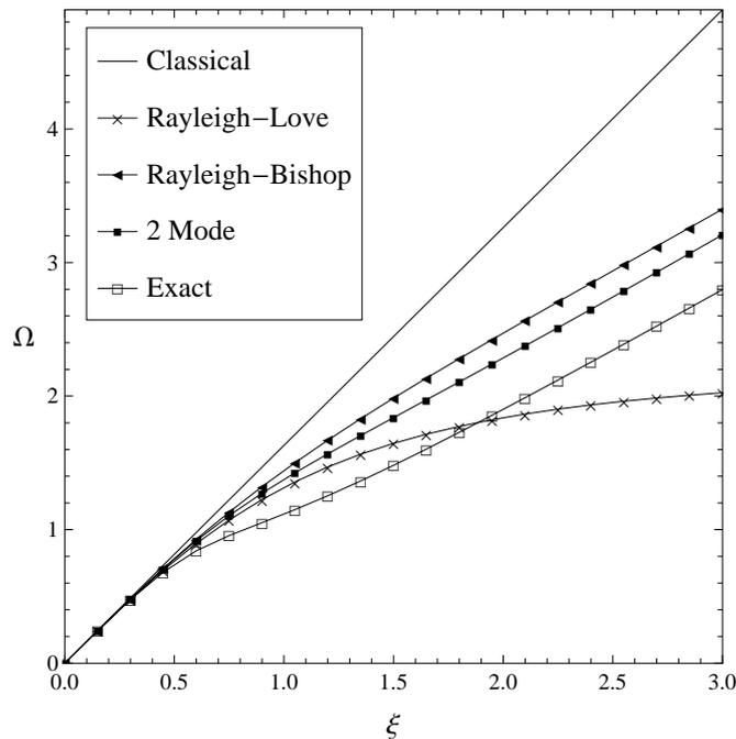
Figure 1: Frequency spectrum of the classical, Rayleigh-Love, Rayleigh-Bishop, two mode (first branch) and exact (first branch) theories.
